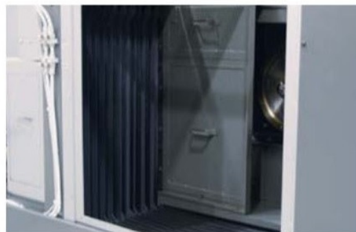
High Visibility skeleton cover Monitoring of wheelhead motion is possible from outside of the cover.
